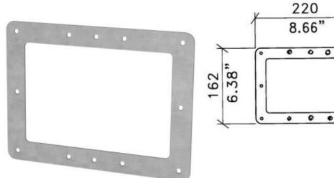
FIXING HOLES 5mm /.20"DIA
